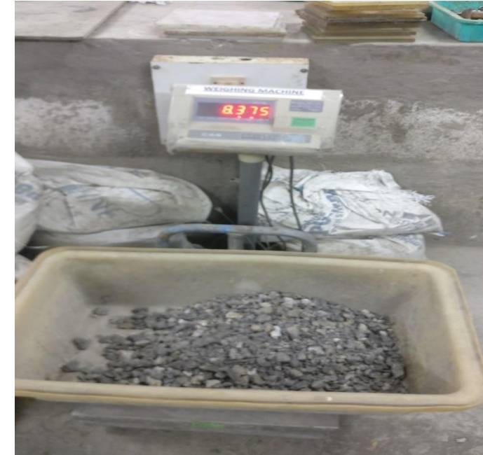
Weighing ingredients according to mix design
